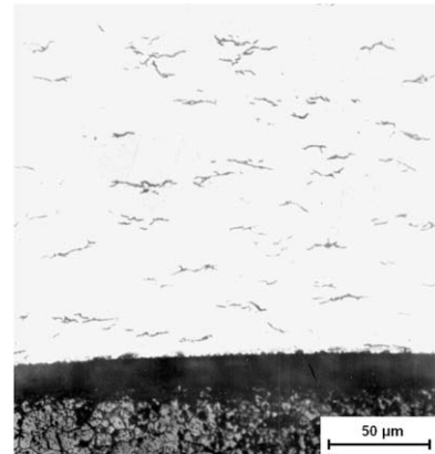
Fig. 5. Sheath hydriding features.
